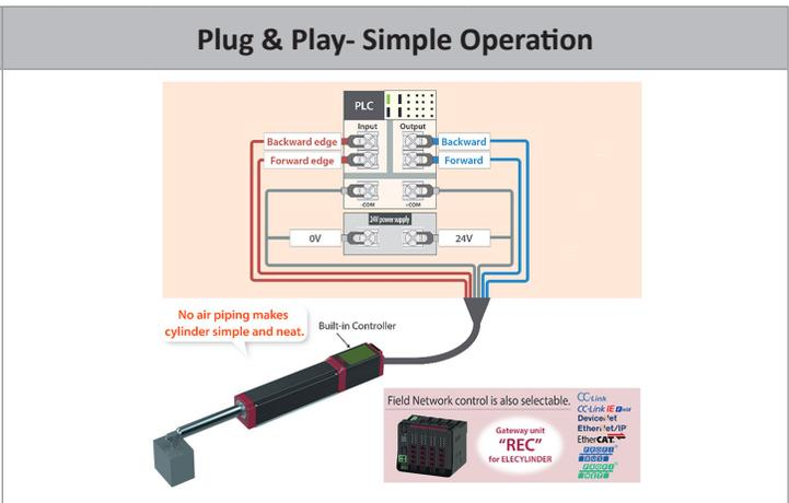
Actuator has built-in motor and drive. Only requires connection of 2 Cables (communication cable and power cable).
